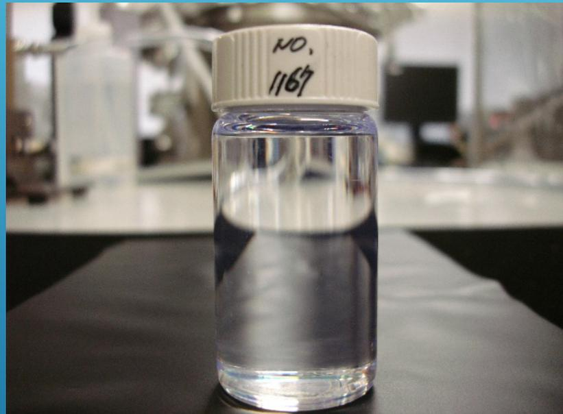
**> 70g/L of Zirconium could be solved in anisole.**
