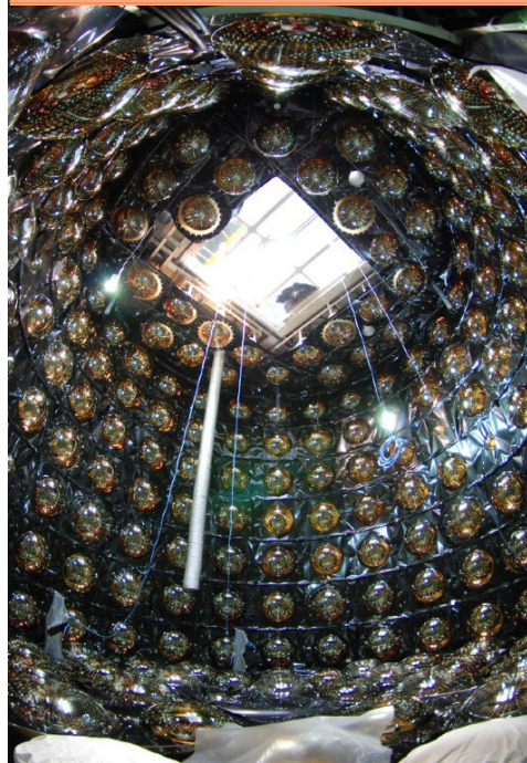
200 m 3 tank with 240 PMTs
