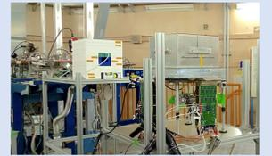
Measure the  $\gamma$ -rays BG from laboratory via  $(n, \gamma)$  reactions
