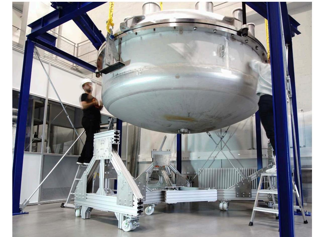
Test electrodes with 2.6 m diameter: U. Freiburg
