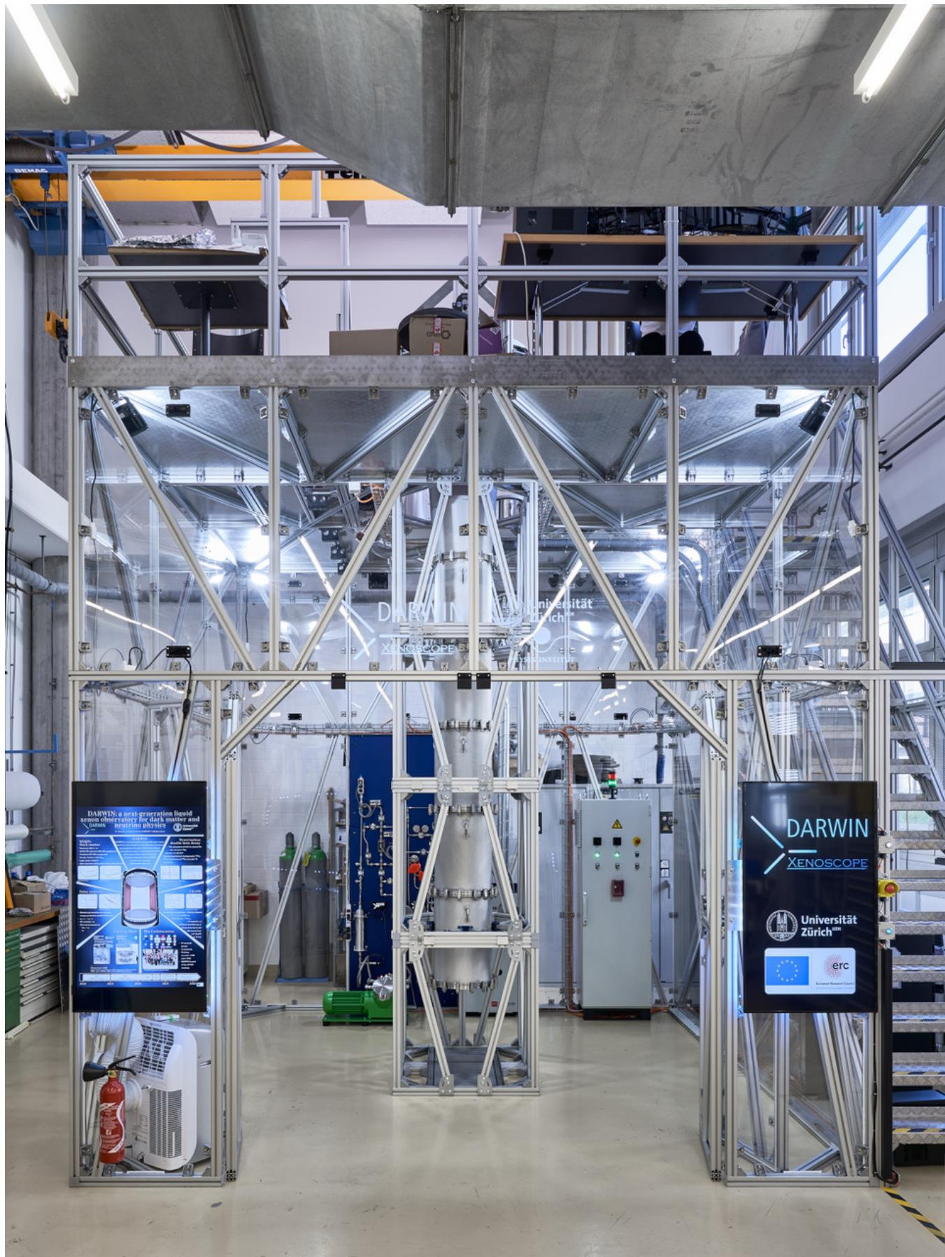
Test e<sup>-</sup> drift over 2.6 m (purification, high-voltage): U. Zurich
