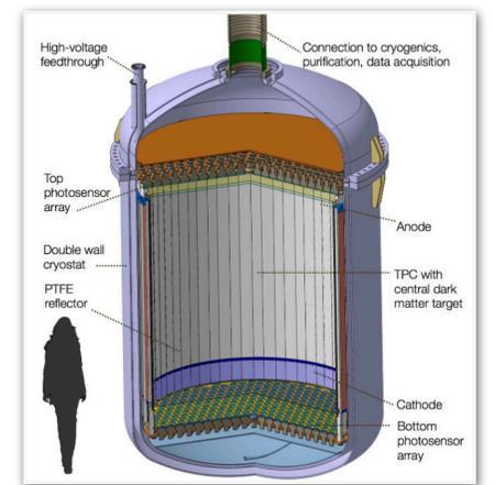
**Multi-ton scale liquid xenon/argon experiments**
