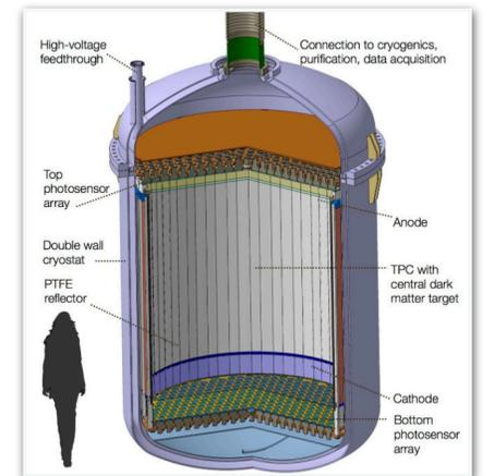
**Multi-ton scale liquid xenon/argon experiments**
