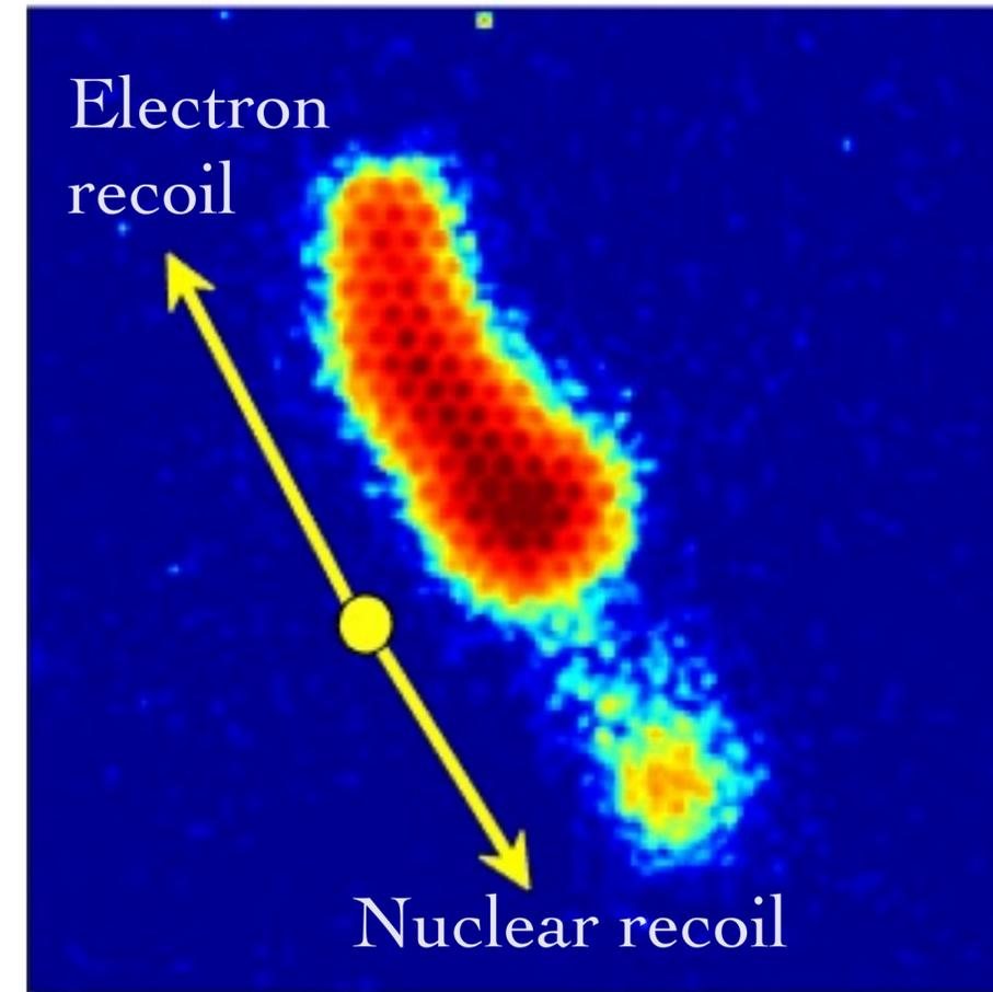
Could be confirmed directionally, using a small-scale optical TPC -
