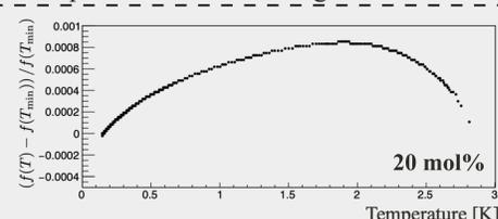
One resonant frequency shift over temperature
