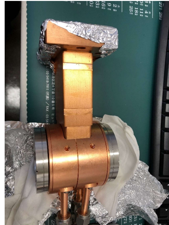
Pre accelerating cavity 5.712 GHz single cavity Max. 100 kW
