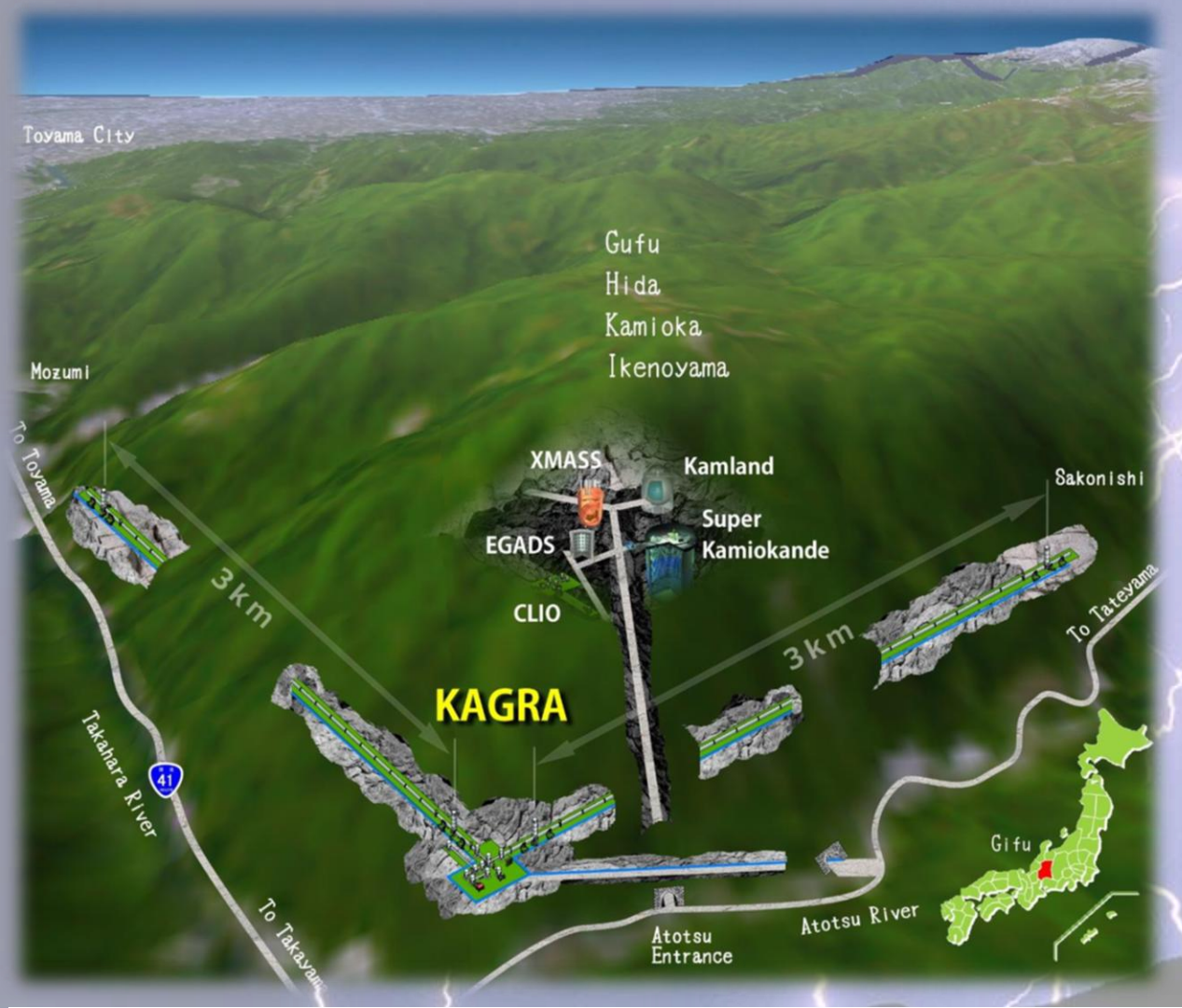
The laser interferometric GW detector constructed at Kamioka underground (200~450 m)
