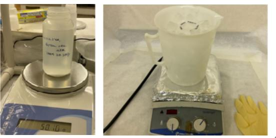
**2. Chemical separation of <sup>226</sup>Ra** Extract Ra ions using AnaLig® Ra-01. Elute Ra ions by EDTA solution.
