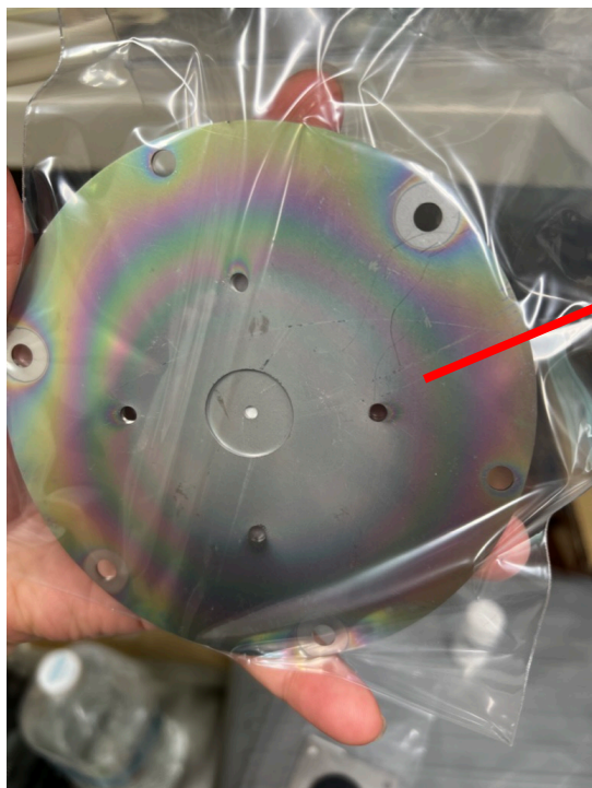
∅120 mm SUS304 Collection plate (Max temperature = 700°C)
