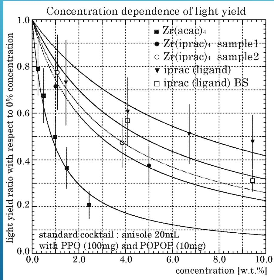
Light yield of  $\text{Zr(iprac)}_4$  even with small bump recovered about double compared with  $\text{Zr(acac)}_4$ .
