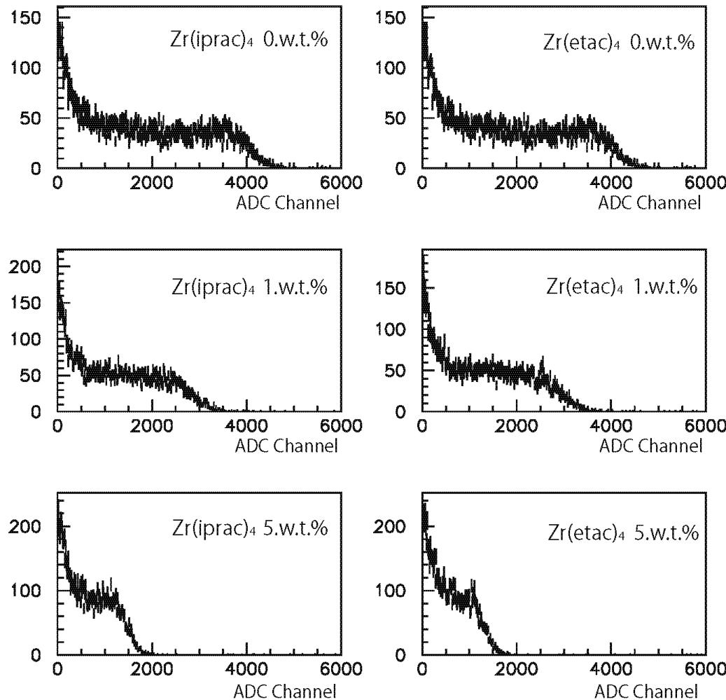
Light yield decreased as increasing the concentration of the complex even though small overlapping between the absorption of ligand and the emission of anisole .
