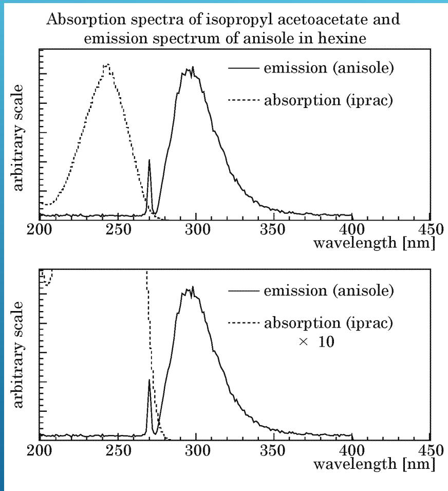
Absorption tail of  $\beta$ -keto ester ligands slightly overlapped with the region of the emission of anisole.
