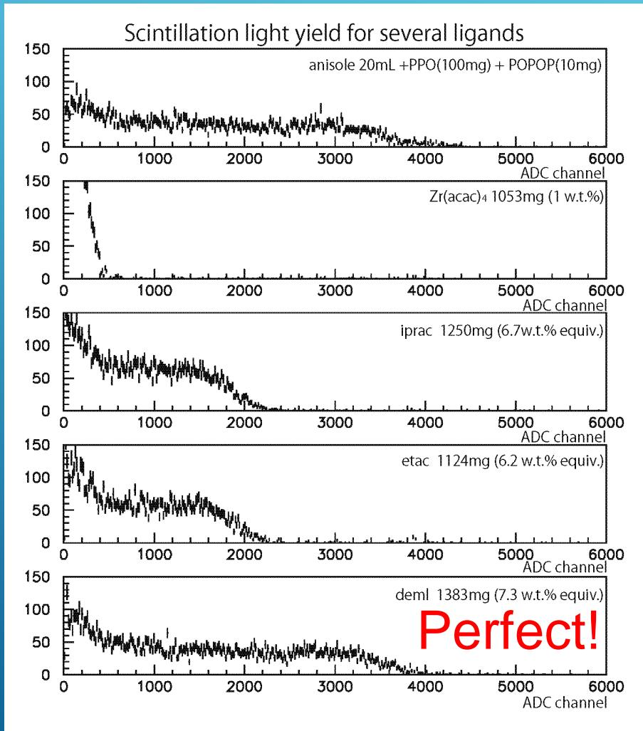
No quenching due to overlap between the absorption of ligand and the emission of anisole should be occurred.
