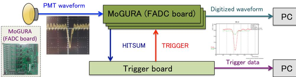
1. Scintillation light is detected by PMTs and its waveform is digitized by MoGURA.
