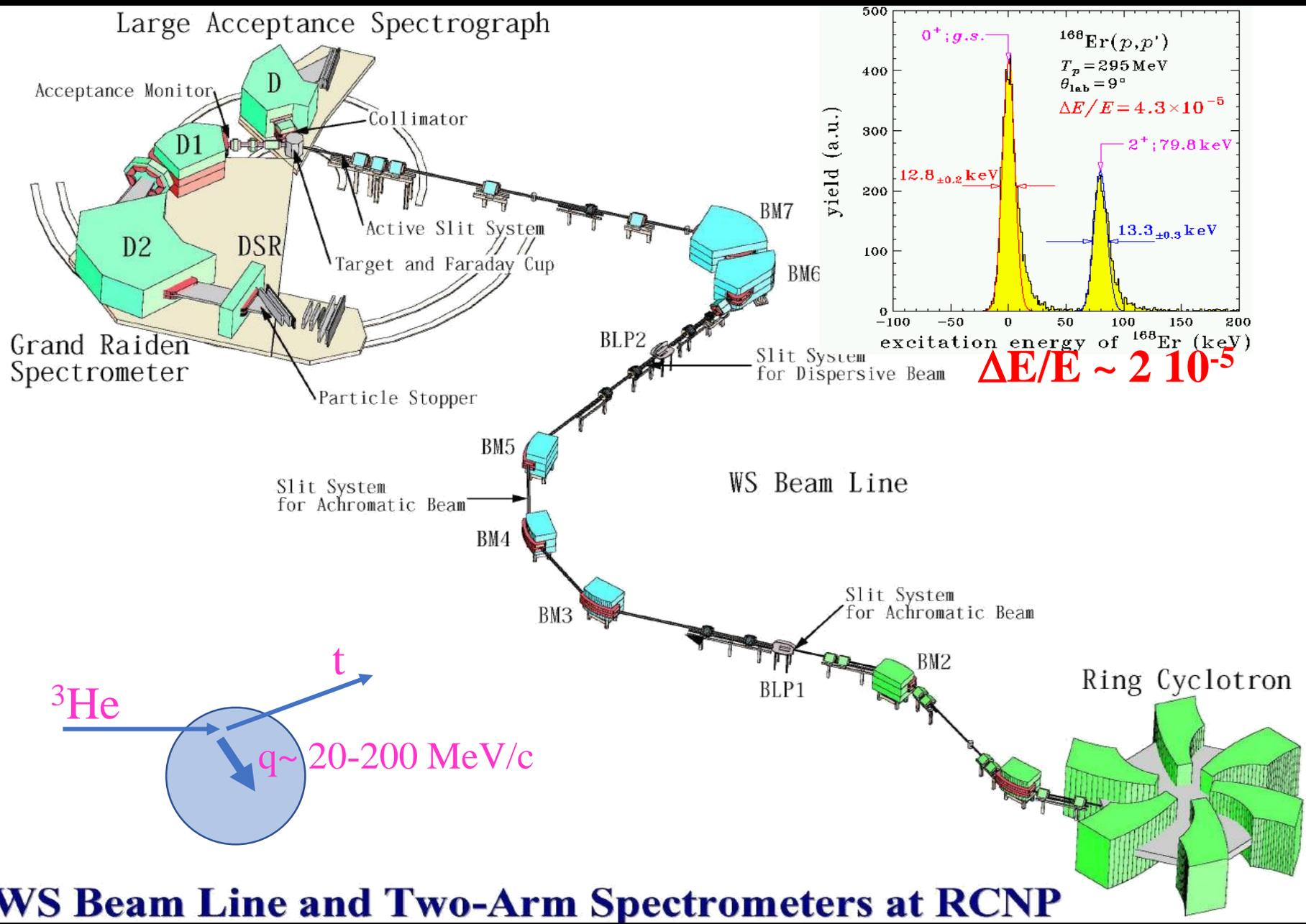
**WS Beam Line and Two-Arm Spectrometers at RCNP**
