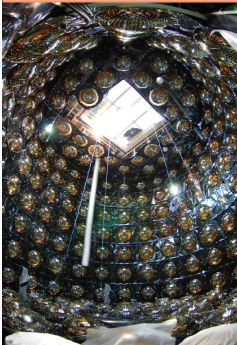
200 m 3 tank with 240 PMTs
