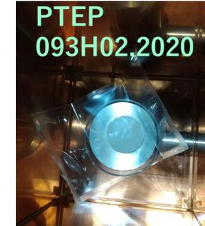
Ra captured resin disk after Gd sulfate solution passed
