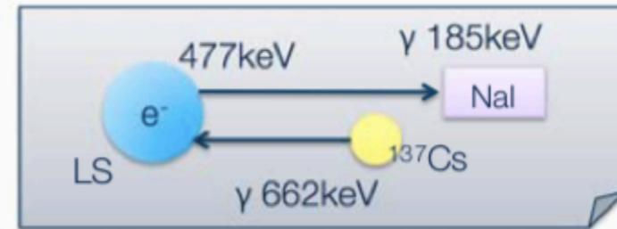
Due to setup, measurement is not back scattering ( $\theta = 180^\circ$ ).
