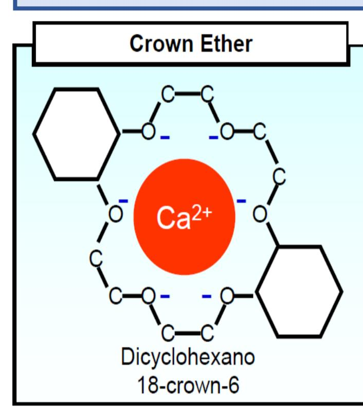
Hold by electrostatic attraction between Oxygen atoms (negative charge) and cation ( $\text{Ca}^{2+}$ )
