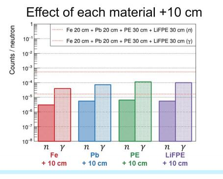
When increasing the thickness of only 1 of the 4 materials, Fe gave the most effective enhancement in shielding.
