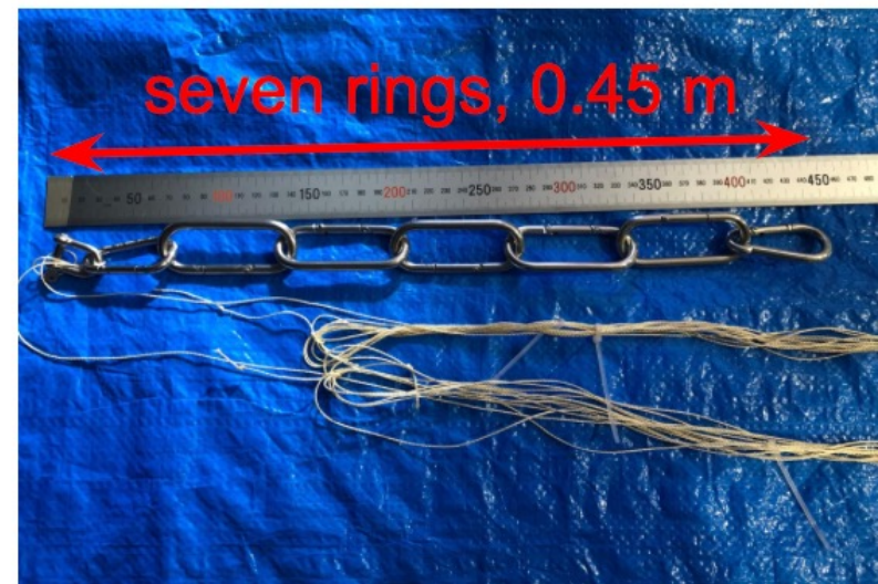
Installed chain and vectran
